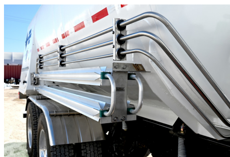
Pressure building unit and hydraulic lines
